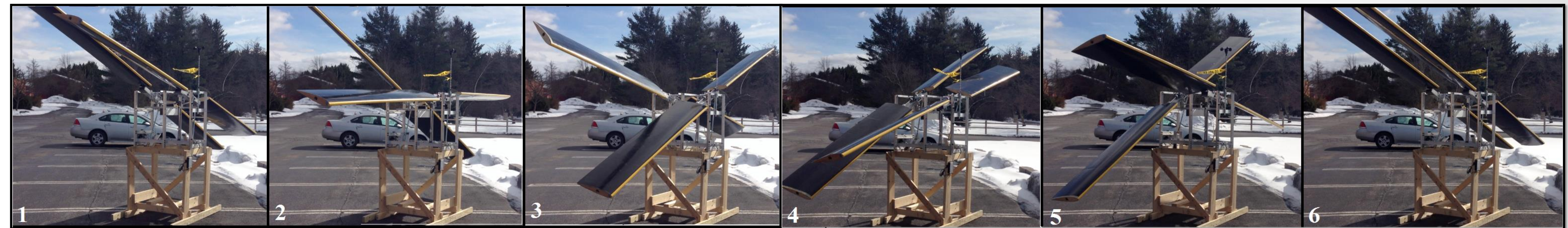
Fig. 3 – Motion of the wing mill through one cycle. – [1] The wing mill begins with slightly pitched wings and the wind pushes the front wing downwards [2]. Once the wings have reached the bottom of the cycle [3], the wing pitches are reversed to create lift [4,5] and move back to its original position (6). The rear set of wings is 90 degrees offset from the front set.
